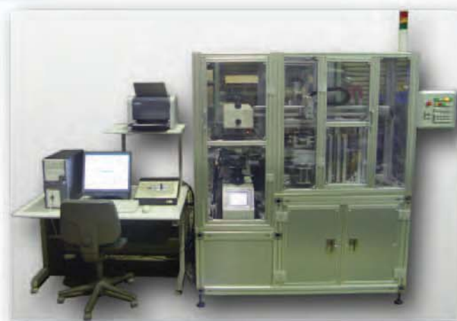
写真は、試験品の供給、排出、研磨も含めたフルオートシステム The fully automatic system which included supply of specimen, ejection, polishing
