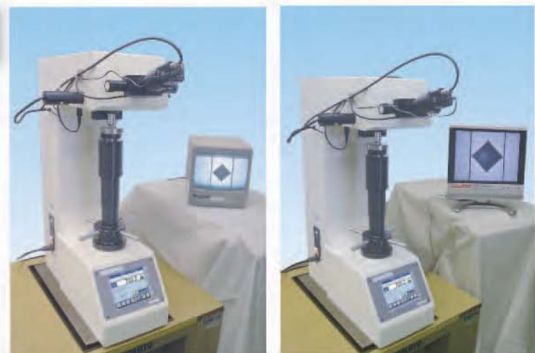
TV計測装置CRTタイプ縦型(型式: CRT1) TV計測装置LCDタイプ縦型(型式: CRT1L) CRT type, Vertical type attachment(model: CRT1) LCD type, Vertical type attachment(model: CRT1L)
