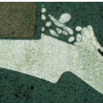
Weld structure, brightfield
