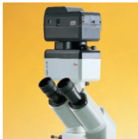
Trinocular tube HC ILT with MPS30
